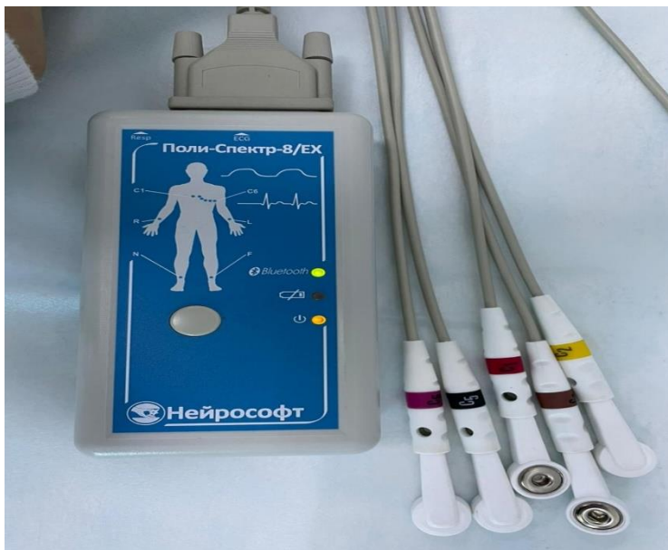
Figure 1. Device for determining heart rate variability “Poly-SPECTRUM” from Neurosoft
